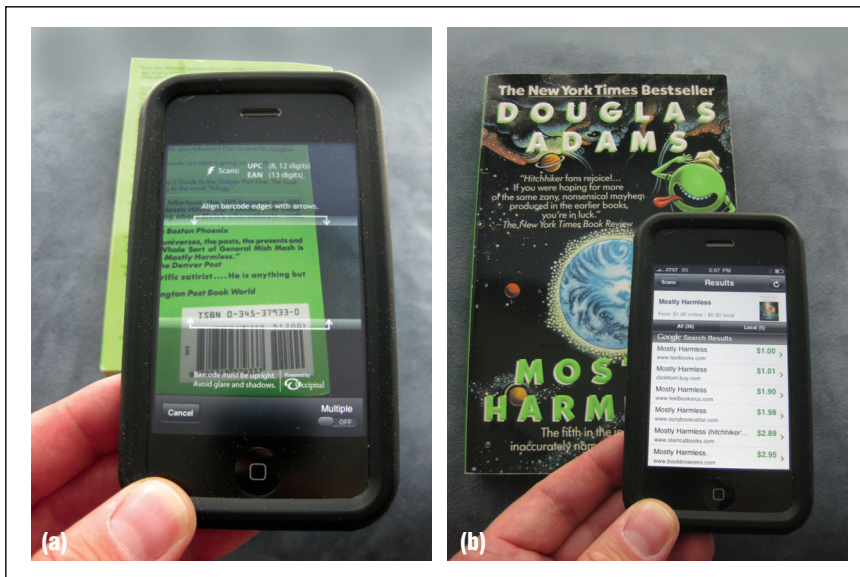
Figure 2. RedLaser. (a) The user positions the camera recognition system over a bar code on the back of a book. (b) A moment later, RedLaser recognizes the book's bar code, links to online data, and provides a list of links to vendors.
