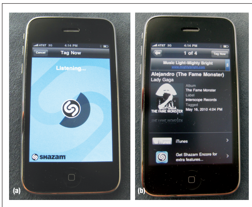
Figure 4. Shazam. (a) The app listens to a song on a nearby radio. (b) After 10 seconds of listening, the Shazam online service analyzes the song and presents details.
