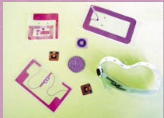
RFID Tags in Various Shapes and Sizes
